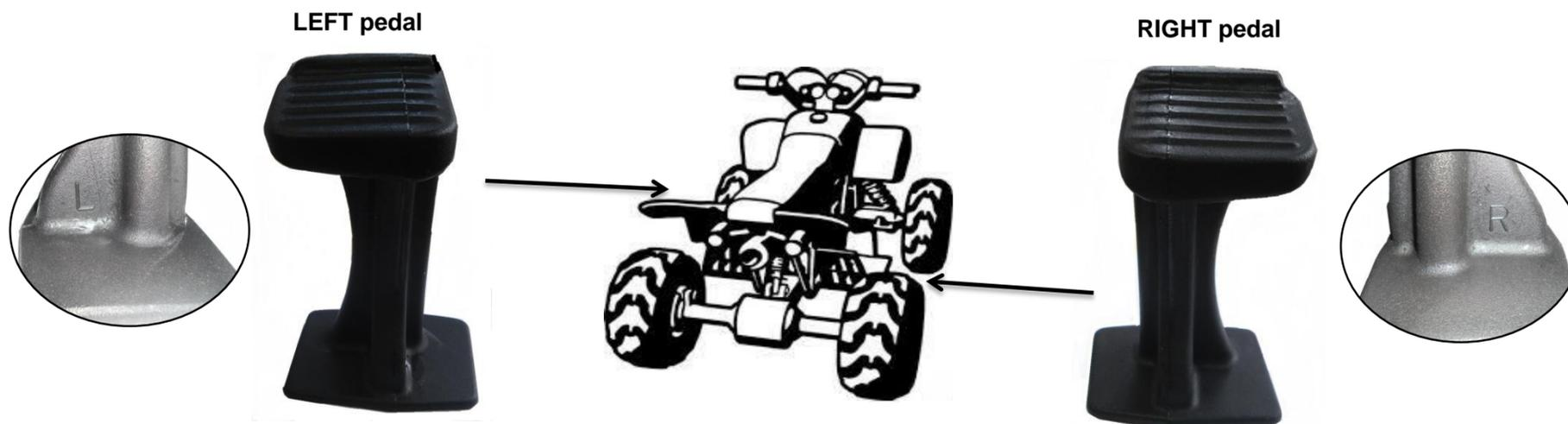
**Step: 2** Place each foot pedals on the ATV's footrests and fix them securely as shown here:
